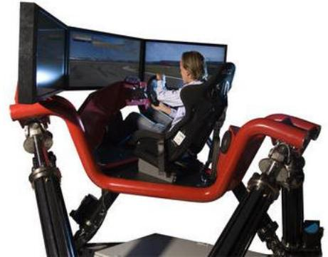
The Simulator company Cruden has built an F1 simulator that costs a hefty £120,000. The simulator is called the Hexatech and is capable of providing 6DOF (six degrees of freedom).
