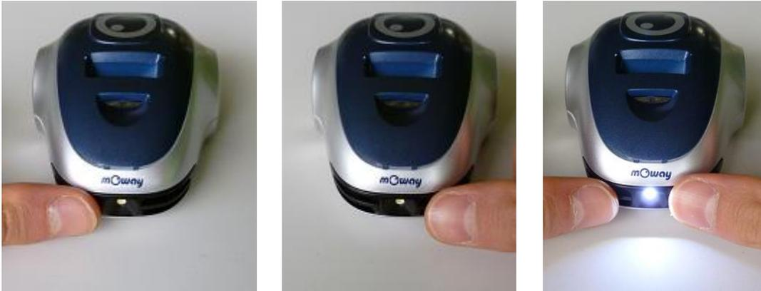
However, if you choose the **OR** option, the output of the block will be true when **ANYONE** of the conditions is met. For example, if you activate the two obstacle central sensors and tick the OR checkbox, the output will be true when either the left central sensor detects an obstacle **or** the right central sensor detects an obstacle.
