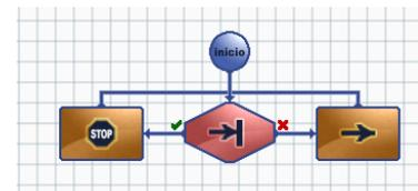
We have just created a **loop**. The robot will perform the same program over and over and check for any obstacle.
