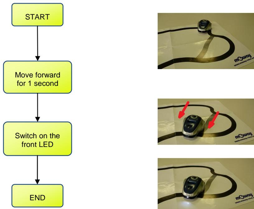
This way to represent programs makes it much easier to understand, especially in the case of complex programs, with a number of actions. The actions to be performed (and their order) can be seen and understood at a brief glance.
