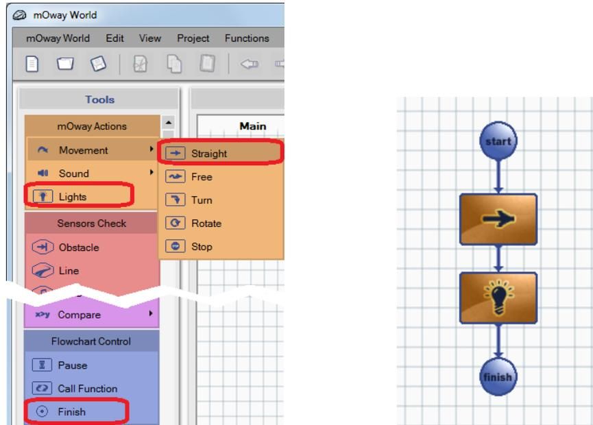
The configuration of the “Movement -> Straight” and “Lights” blocks is as follows:
