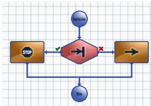
That is, the **condition** needed for the robot to stop is that its obstacle sensors detect an obstacle in front of the robot.
